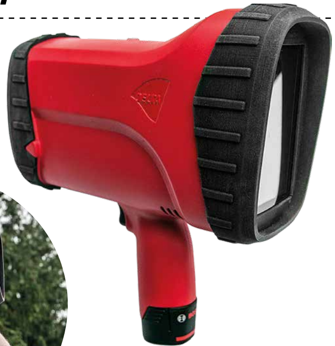
(Above and left) The new RetroSign GRX can capture seven observation angles in a single measurement
